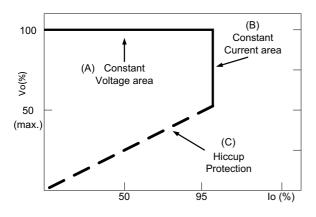
Typical LED power supply I-V curve
