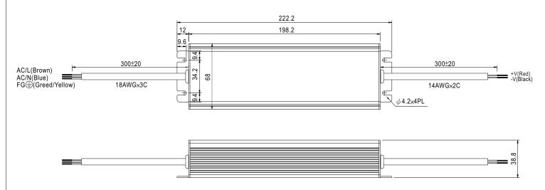
%IP67 rated. Cable for I/O connection.
