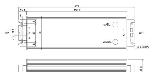
Output voltage and constant current level can be adjusted through internal potential meter. (Can access by removing the rubber stopper on the case.)
